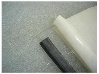
5. Again, incise the extrusion no less than 1-1/4" from the end of itself and slice the bottom layer off.
