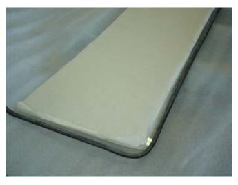
4. Cut the material, as was done on the other side, at a distance 3/8" from the bottom of the shield. Set the remaining length of extrusion aside for the bottom of the shield in the upcoming steps.
