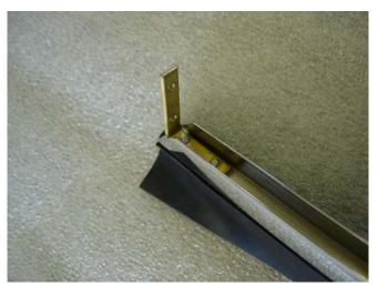
3. Now remove the upper loop of the windshield frame from the glass; spread the sides first, then remove from the top. Use the block of wood and hammer if necessary. After the glass is removed, thoroughly clean the channel of the windshield frame with mineral spirits or paint thinner.
