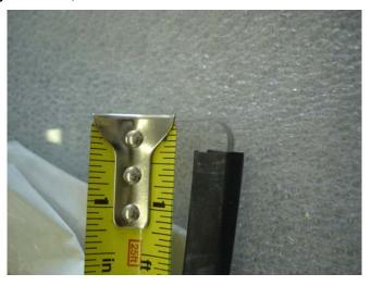
2. Make an incision into the gasket at a distance no less than 1-1/4" from the end of the extrusion (i.e. 1-5/8" from the bottom of the shield). Now slice the bottom of the gasket off, up to the incision mark as shown below. These cuts allow clearance for the brass angles within the channel of the frame.
